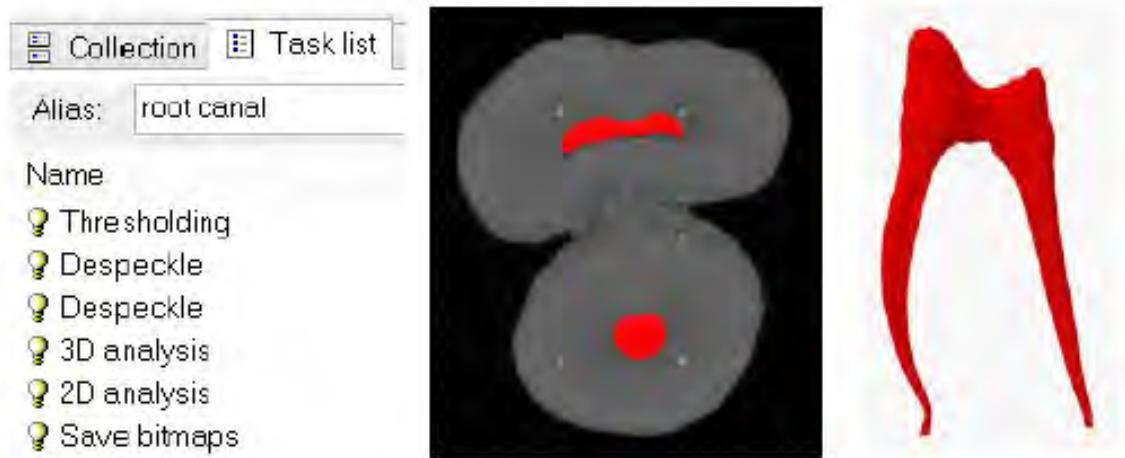
Figure 6. The collections tab allows often-used task lists (e.g. “root canal”) to be available for quick access.
